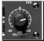
The Output control is used to set the desired output of the Blue Max. It is sometimes referred to as 'gain makeup' control. This terms is derived from the fact that as the compressor lowers the output level during gain reduction, the overall signal level is lowered, requiring the user to 'makeup' the gain thereby restoring the original signal level.
